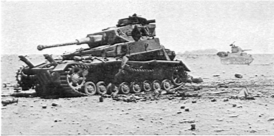
This PzKw IV fared badly, despite its 7.5-cm KWK. Its muzzle brake is the first 7.5 pattern with a single baffle only. Later versions noted in Tunisia have the double baffle effect, patterned after the original brake on the PAK 38.
