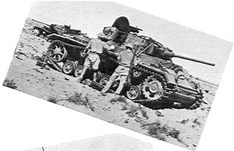
This PzKw III carries the long-barrelled 5-cm KWK (Kampfwagon Kanone). Tube of this gun is almost identical with that of the PAK 38. Both pieces use the same ammunition except for the primer; with the PAK this is percussion, but the KWK uses an electric one. Cans with white crosses are water cans, embossed Wasser on their sides; similar cans without crosses are for gasoline, and are embossed Kraftstoff.
