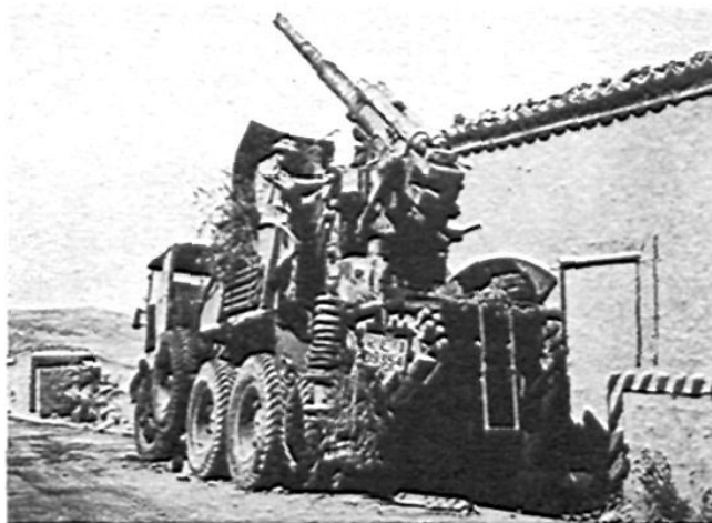
Among Sicilian booty was this Italian Ansaldo 90/53 gun, Model 41, which in 1942 had been mounted on a Lancia heavy-duty Diesel-powered cargo truck.
