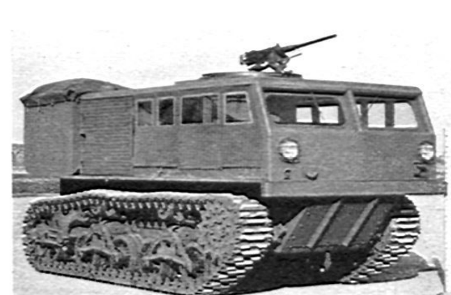
M4 tractor is for the 155-mm gun, 8" howitzer, and the modified 240-mm howitzer. It too will carry a small amount of ammunition, in addition to crew and section equipment.
